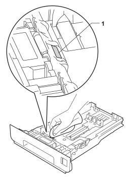
Wipe the two pick-up rollers (1) inside of the machine to remove dust.
